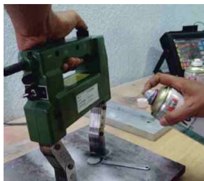
NDT Check of Welding
