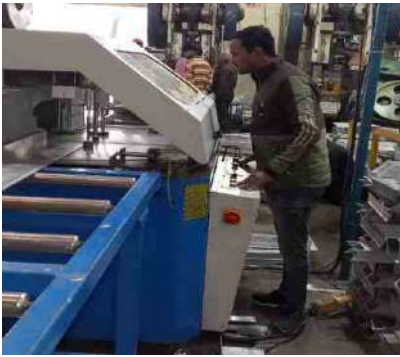
Cutting of Sections by Automatic Angular Cutting Machine
