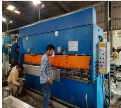
Hole Punching by PLC control Automatic machine
